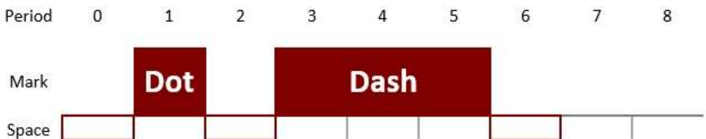
Figure 2 Timing diagram for the letter A in Morse code, an element of 6 dot-lengths
